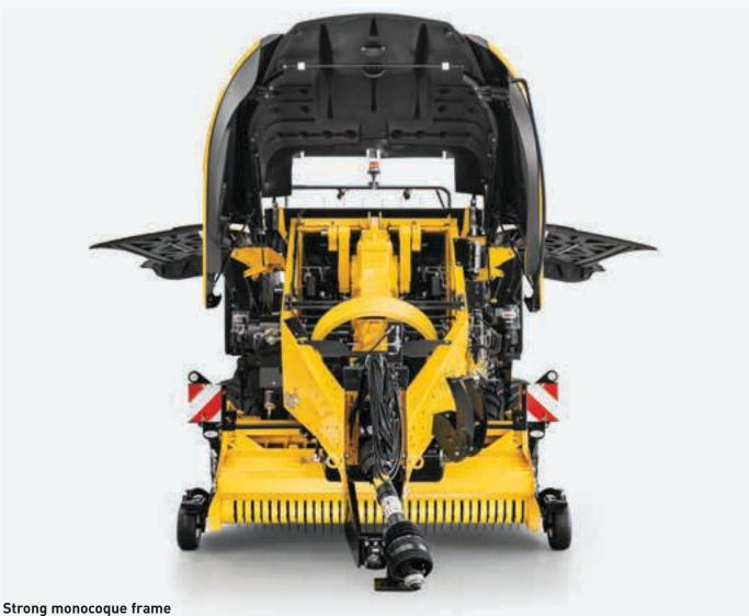
•The single piece frame has been engineered to offer outstanding structural strength for enhanced reliability and reduced vibration
